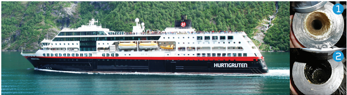
1. Hard urine scale in MS Midnatsol's piping was a problem. 2. Treatment with Jets™ Descale Plus proved very efficient.
